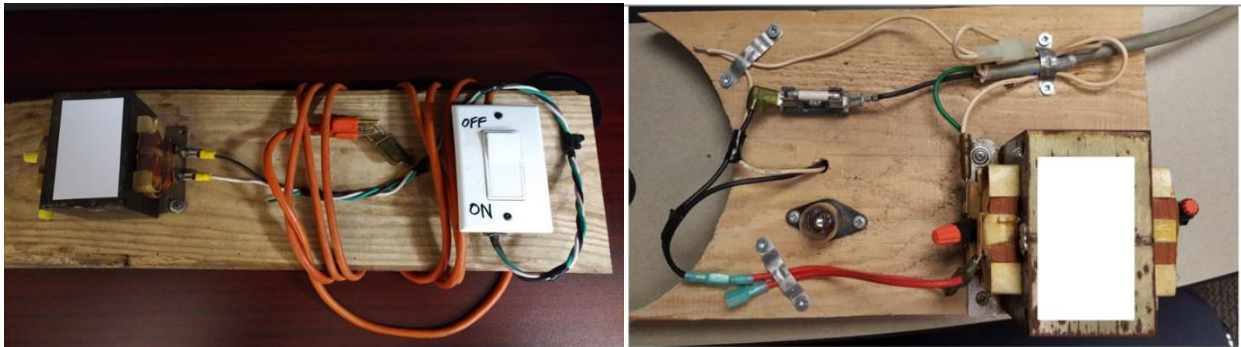
Pictures 2 and 3 - Examples Of Homemade Lichtenberg Generators
